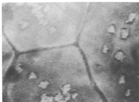
Figure 2 White light image of 30 kg indent region showing mapped area.
